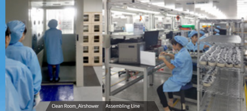
Clean Room_Airshower Assembling Line
